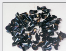
Chip feature after drilling
